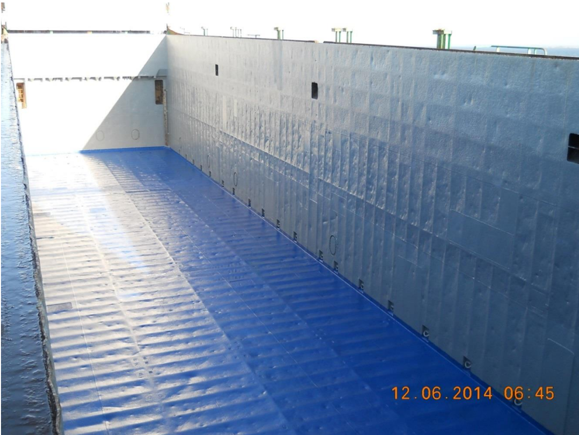
Cargo hold seen from aft to fore – no narrowings
